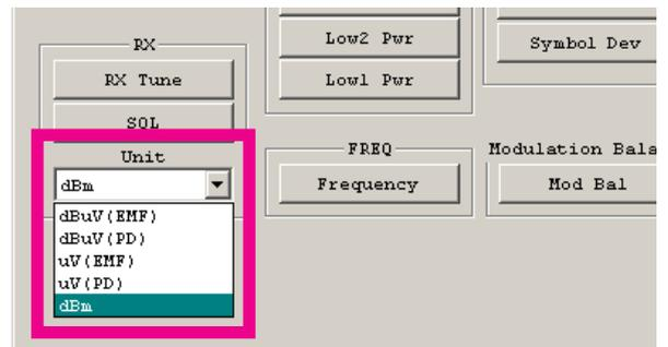
When perform the RX Tune and SQL alignment, the RF level shows this unit according to this setting.
