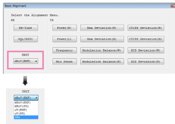
When perform the RX Tune and SQL alignment, the RF level shows this unit according to this setting.
