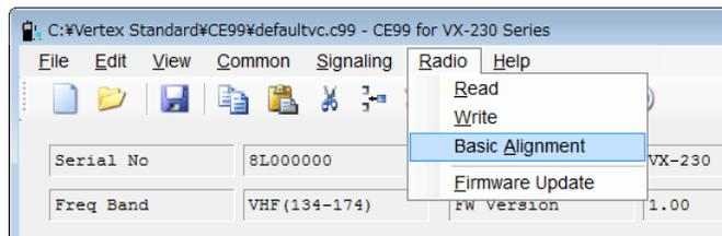
To enter the Basic Alignment Mode, select “Basic Alignment” in the main menu “Radio”. It will start to “Read” the written personalized data from the radio. Then pressing the button “OK” will start the Basic Alignment Mode.
