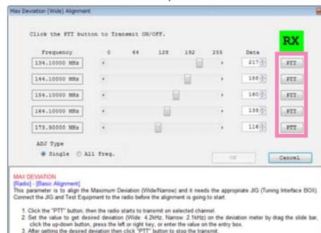
You may select the alignment type from the Radio button (ADJ Type) located at the bottom of the screen, as needed..
